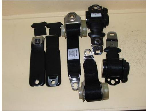
Look at that. Absolutely stunning work. It will be a pity to put them under covers under the seats. The latches were re-chromed and all the parts within the mechanism were checked for deterioration and replaced if needed. They even cleaned the original tags and put them on the new belt webbing.
